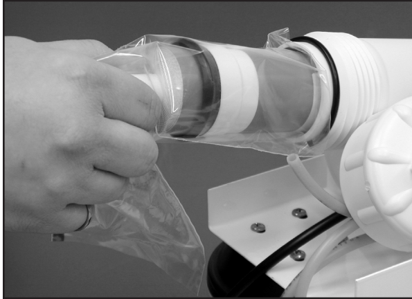
Figure 8 - Installing membrane without touching
