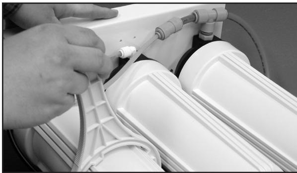
Figure 11 - Using sump wrench to change filter cartridges
